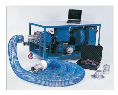
Dresser's 20M/5M Model 5 Prover is the newest addition to the Model 5 ROOTS® prover family of transfer provers. The cart-mounted prover gives you the increased capability to prove rotary, turbine and diaphragm meters up to **20,000 acfh**, while occupying minimal floor space.
