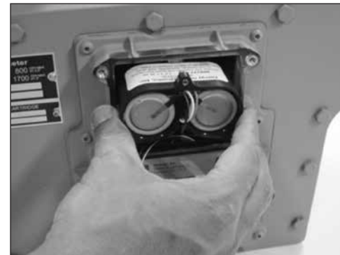
Figure 9.22 - Place battery inside compartment
