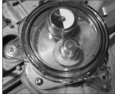
Figure 9.40 - Place O-ring on amber cartridge cover
