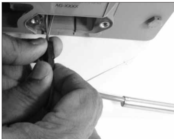
Figure 9.3 - Press and release the black connector to remove temperature probe
