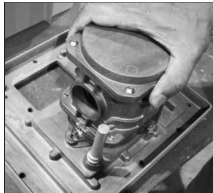
Figure 9.41 - Proper alignment of measurement cartridge
