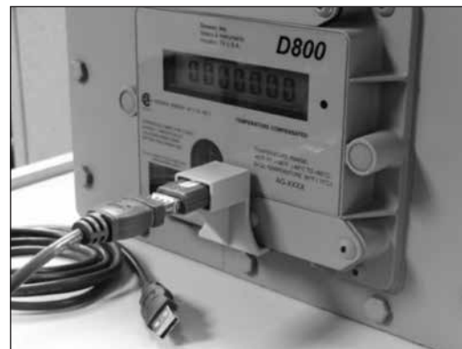
Figure 12.1 - Proper Installation of IrDA cable to the meter
