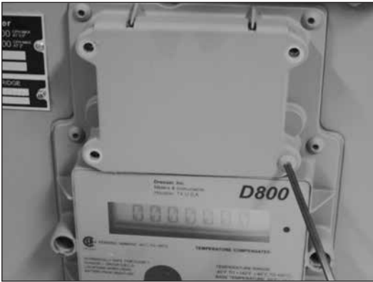
Figure 9.7 - Remove 4 screws on battery compartment
