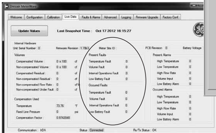
Figure 8.2 - Live Data Screen showing Faults in Dresser MeterWare Software
