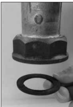
Figure 7.1 - Proper installation of washer into swivel
