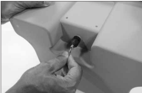
Figure 9.26 - Push pulse output cable back into the meter
