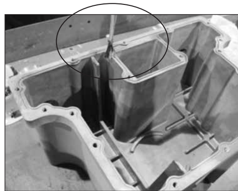
Figure 9.45 - Apply grease to rear enclosure
