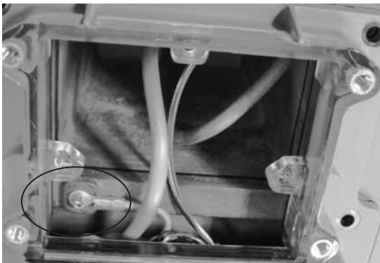
Figure 9.19 - Attach green ground wire
