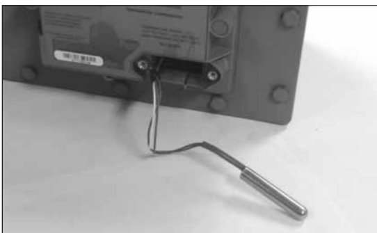
Figure 9.20 - Temperature probe extended through the front of the instrument cover
