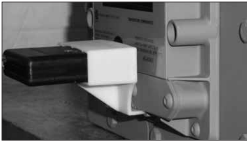
Figure 10.15 - IrDA adapter placed into slot
