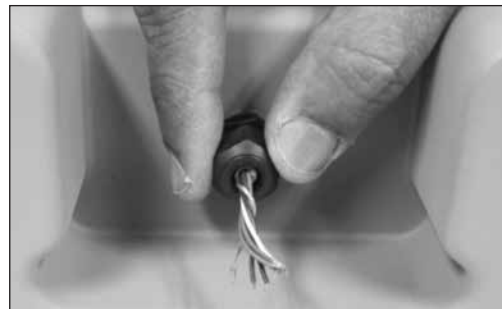
Figure 9.11 - Loosen cable gland connector
