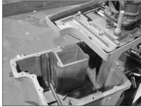
Figure 9.35 - Front enclosure removed
