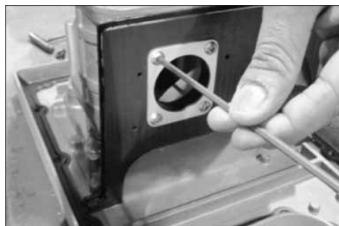
Figure 9.37 - Remove 4 (#10-24) screws on main gasket
