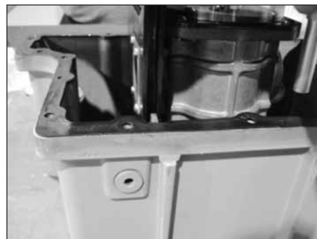
Figure 9.47 - Aligning gasket slots with ribs
