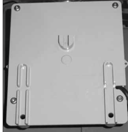
Figure 7.23 - Attach ERT to backplate with Torx screws
