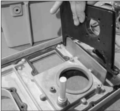
Figure 9.39 - Remove main gasket
