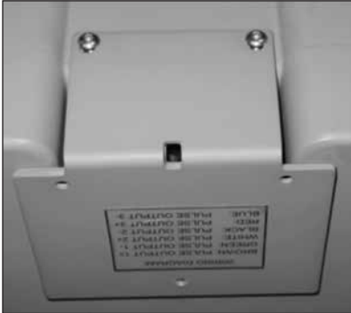
Figure 7.14 - AMR mounting brackets as shipped from factory
