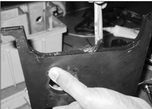
Figure 9.43 - Apply grease to gasket
