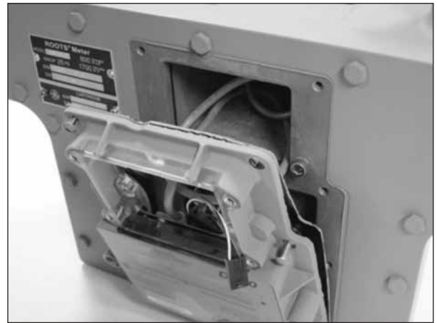
Figure 9.9 - Pull index away from the meter
