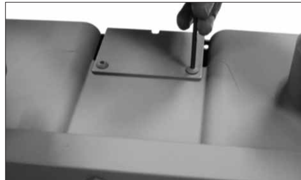
Figure 9.27 - Attach AMR plate to the meter.
