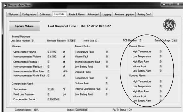
Figure 8.3 - Live Data Screen showing Alarms in Dresser MeterWare Software
